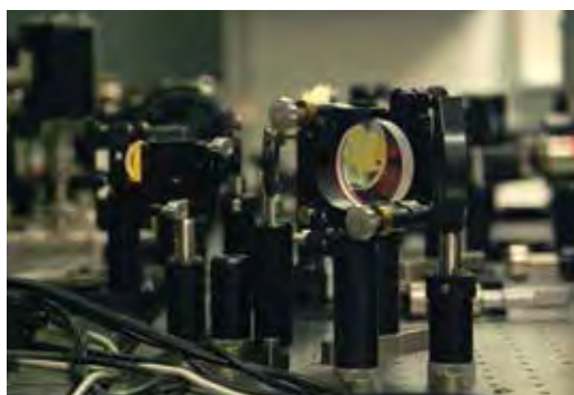
PHOTOS FROM LEFT: PRECISION OPTICS RECOMBINE OPTICAL CENTRIFUGE PULSES. THE GREEN LIGHT AMPLIFIES THE POWER OF THE PULSES. THE EXTREME ROTATIONAL STATES OF N 2 O ARE CREATED AND PROBED IN A LOW PRESSURE CELL.
